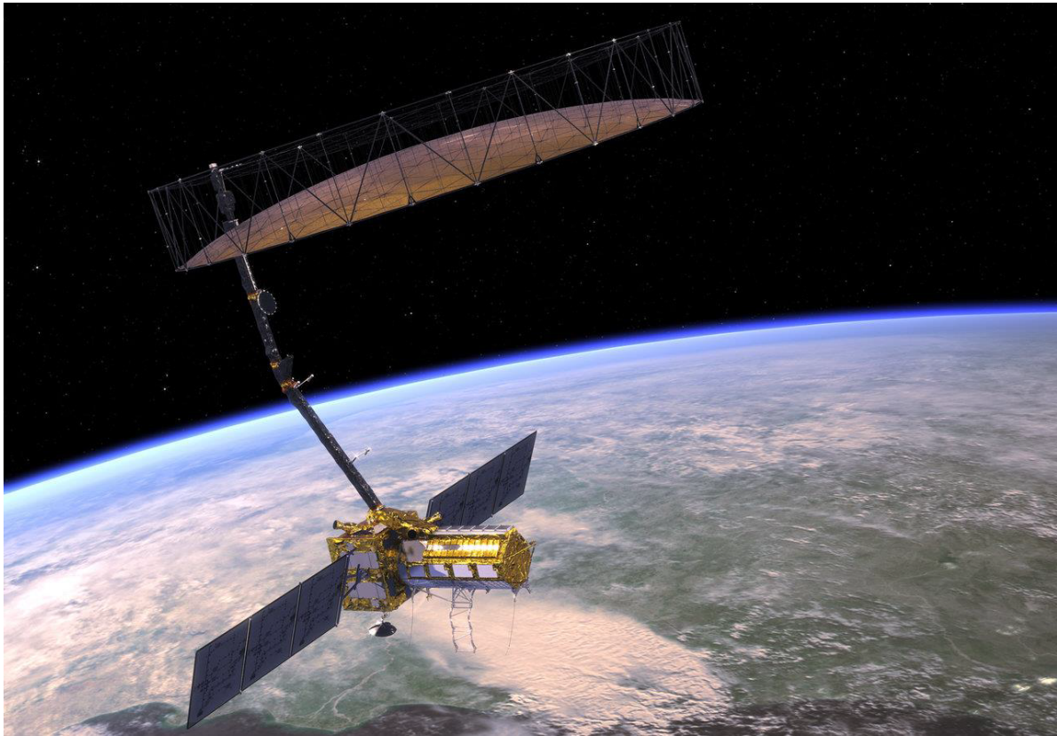
Figure 21: NISAR spacecraft rendering showing the large deployable L-band antenna (12-meter diameter) and S-band antenna. The mission will provide systematic global SAR coverage every 12 days with full polarimetric capability at L-band. NISAR specifically targets ecosystem structure, biomass, and change detection applications, with open data access enabling operational forest monitoring. Source: NASA/JPL-Caltech
